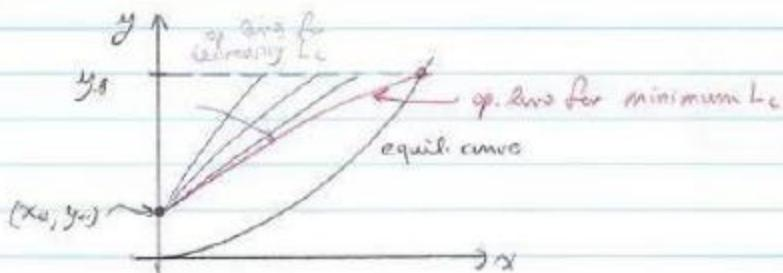
Because equil. curve is concave up, 1<sup>st</sup> contact occurs at "b" end of op. line.  $\therefore$  for minimum liquid
