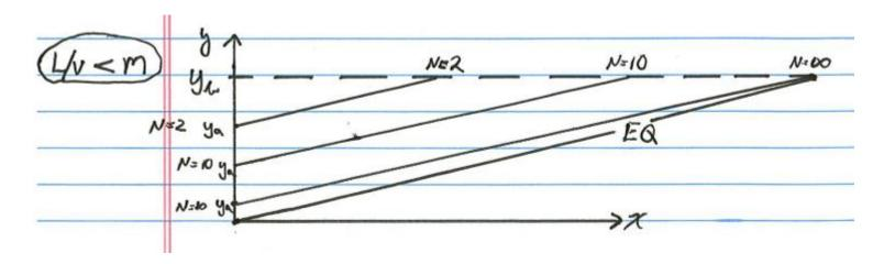
Continuing to add stages will NOT lead to a lower value of y<sub>a</sub>
