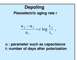
Ferroelectric - A material that shows spontaneous and reversible dielectric polarization. **Piezoelectric** – A material that develops voltage upon the application of a stress and develops strain when an electric field is applied.
