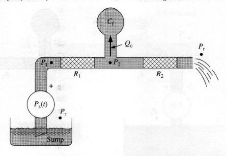
Figure P9.1a First-order low-pass hydraulic filter.
