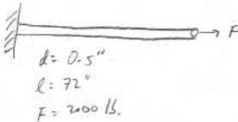
Tensile stress:  $\sigma = \frac{F}{A}$   $A = \pi \left(\frac{0.5}{2}\right)^2 = 0.196$
