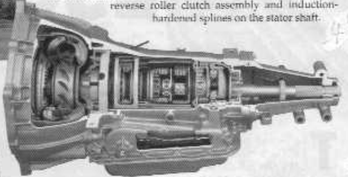
The Escalade's Vortec 6000 engine is linked to a new Hydra-Matic 4L60-E HD (heavy-duty) four-speed automatic transmission upgraded to handle the engine's greater power and torque.
