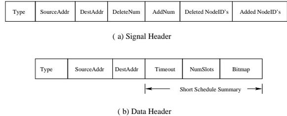
Figure 2: Signaling and data packet header format
