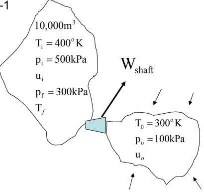
$$\begin{split} W_{shaft} &= m_i u_i - m_f u_f + (m_f - m_i) u_o - W_{flow} \\ W_{shaft} &= 43,554 \text{ kg} \times 287.2 \text{ kJ/kg} \\ &- 30,238.8 \text{ kg} \times 248.2 \text{ kJ/kg} \\ &- 13315. \text{ kg} \times 215.4 \text{ kJ/kg} \\ &- 1,146,435 \text{ kJ} \\ W_{shaft} &= 988,952 \text{ kJ} \end{split}$$
