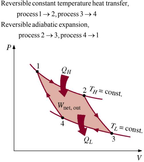
An engineer proposed an attempted to improve the efficiency of a power cycle by transferring heat from the available high temperature source to am alternate higher temperature source using a heat pump. What do you think of this suggestion?
