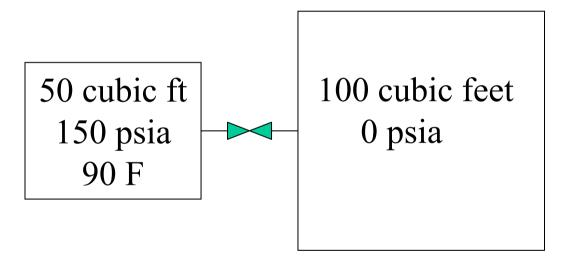
The thermodynamic system is the mass in the pressurized tank. There is no mass in the evacuated tank and thus no system to transfer heat or work to. Neither heat or work are transferred to the system outside the two tanks. Work=0. It is given that Q=0
