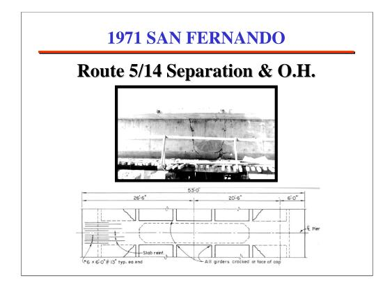
1. Note cracking of incomplete caps, which occurred in Piers 2 and 3. The 45° crack extends through the soffit and exterior girders (slab and soffit only)
