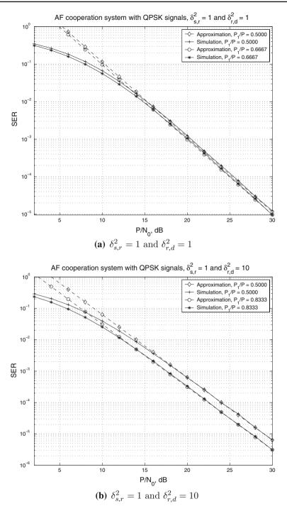
Fig. 8 Performance of the AF cooperation systems with QPSK signals: optimum power allocation versus equal power scheme
