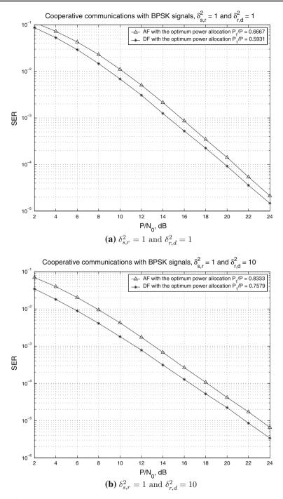
Fig. 9 Performance comparison of the cooperation systems with either AF or DF cooperation protocol with BPSK signals
