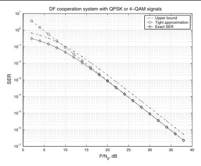
**Fig. 2** Comparison of the exact SER formulation, the upper bound and the asymptotically tight approximation for the DF cooperation system with QPSK or 4-QAM signals. We assumed that  $\delta_{s,d}^2 = \delta_{s,r}^2 = \delta_{r,d}^2 = 1$ ,  $\mathcal{N}_0 = 1$ , and  $P_1 = P_2 = P/2$
