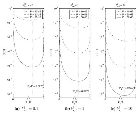
**Fig. 3** SER of the DF cooperation systems with  $\delta_{s,r}^2 = 1$  and  $\delta_{r,d}^2 = 1$ : (a)  $\delta_{s,d}^2 = 0.1$ ; (b)  $\delta_{s,d}^2 = 1$ ; and (c)  $\delta_{s,d}^2 = 10$ . The asymptotic optimum power allocation is  $P_1/P = 0.6270$  and  $P_2/P = 0.3730$ .
