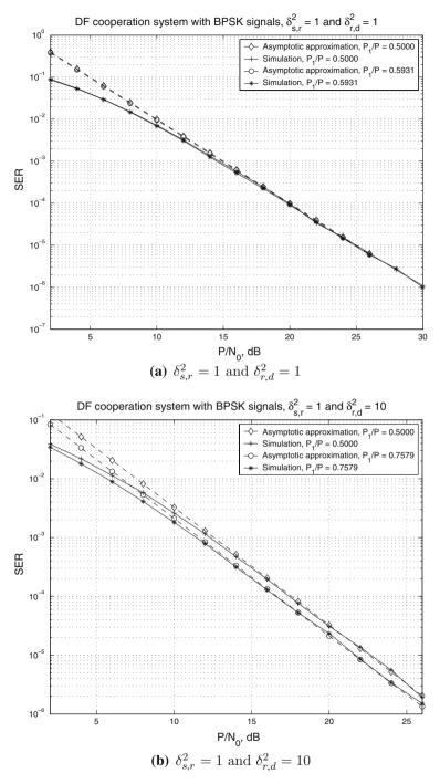
Fig. 5 Performance of the DF cooperation systems with BPSK signals: optimum power allocation versus equal power scheme
