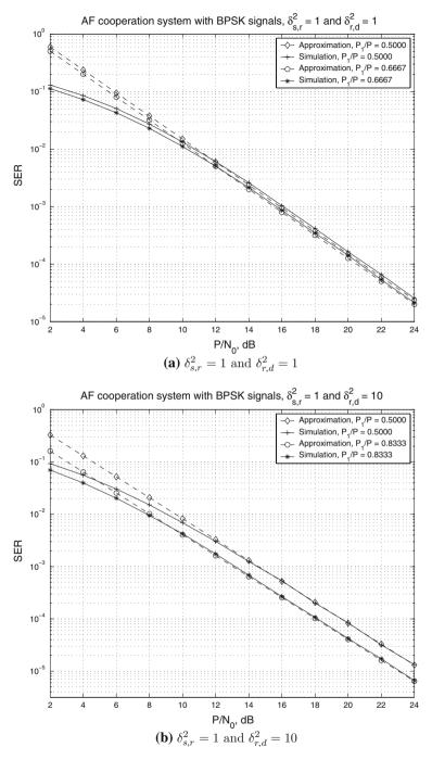
Fig. 7 Performance of the AF cooperation systems with BPSK signals: optimum power allocation versus equal power scheme
