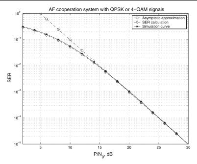
**Fig. 4** Comparison of the SER approximations and the simulation result for the AF cooperation system with QPSK or 4-QAM signals. We assumed that  $\delta_{s,d}^2 = \delta_{s,r}^2 = \delta_{r,d}^2 = 1$ ,  $\mathcal{N}_0 = 1$ , and  $P_1/P = 2/3$  and  $P_2/P = 1/3$
