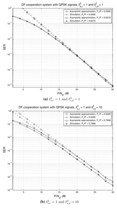
Fig. 6 Performance of the DF cooperation systems with QPSK signals: optimum power allocation versus equal power scheme
