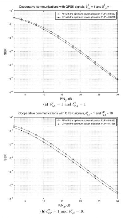
Fig. 10 Performance comparison of the cooperation systems with either AF or DF cooperation protocol with QPSK signals
