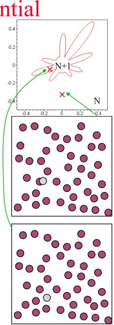
• Widom method is an example of a free-energy perturbation (FEP) technique
